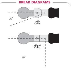
MTBN2 and MTBN10 are supplied with a removable collar, which restricts the "break" angle to  $20^\circ$ . If the collar is removed, the "break" angle increases to  $90^\circ$ .
